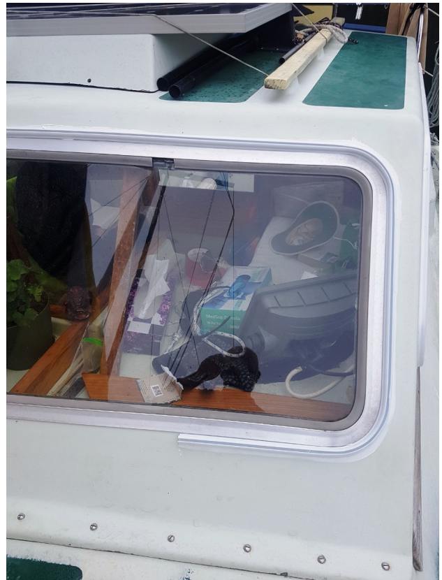
The C-channel PVC bent and fastened outside the exterior window frame.
