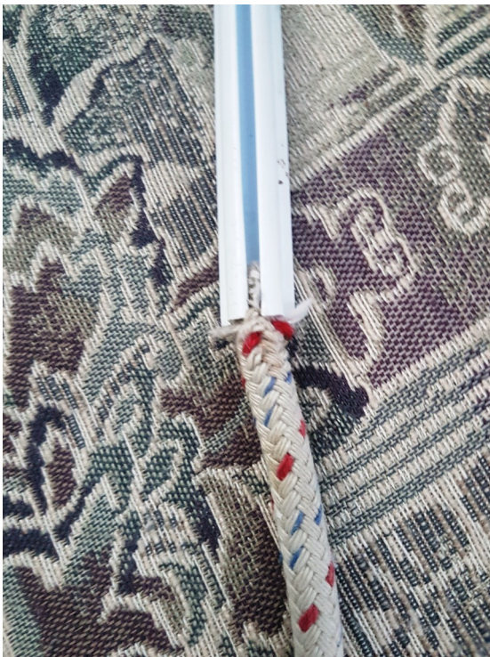
Double-braid rope prevents the C-channel from collapsing when bent.
