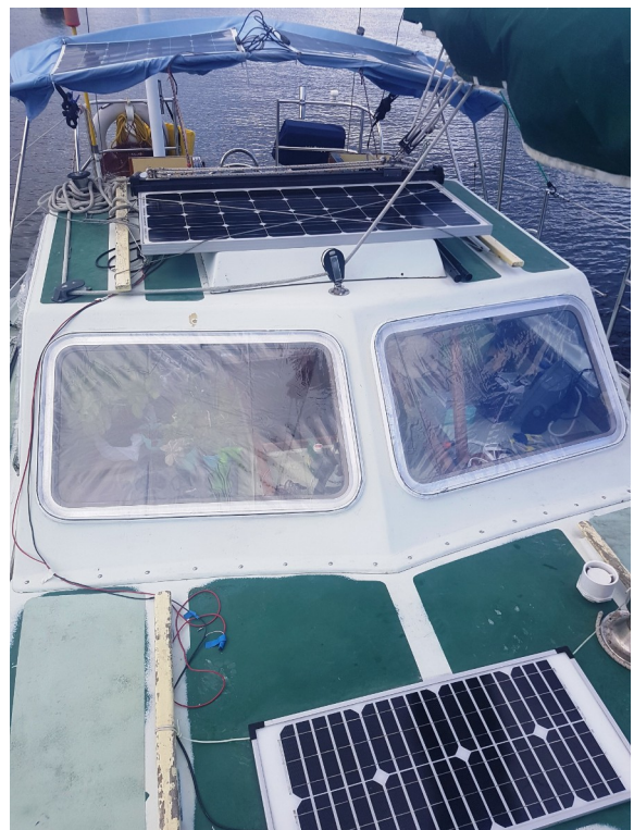
The vinyl is in place with ½-inch DraftSeal backer rod foam tubing.
